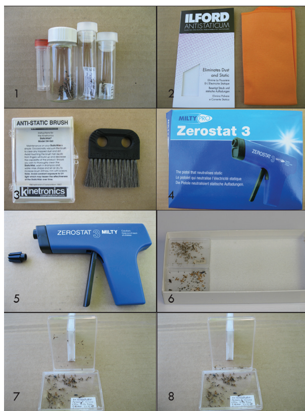
Figures 1–8. 1 Miscellaneous vials for specimen storage 2 Ilford antistatic cloth. 3 Kinetratics antistatic brush. 4 Zerostat 3 product box. 5 Zerostat 3 gun with cap. 6 USNM ½ unit tray with plastic specimen boxes. 7 Specimens attracted to box lid by static. 8 Specimens at bottom of box lid after static dissipated.
